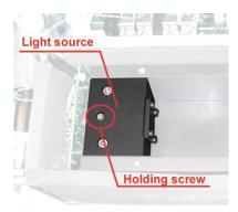
Loosen the screw connector of the lamp's power supply at the pre-amplifier board (labelled: LAMPE)
