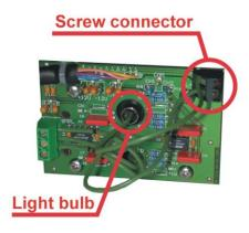
Place a new lamp in the holder and tighten the holding screw
